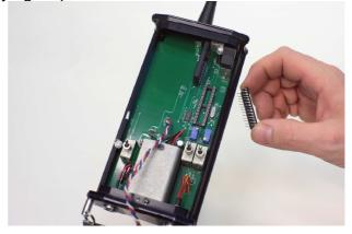
**5.** Carefully install the **BarTech Iris Slider PCB** as shown below into the IC connector of U101. **Note: Board may not be exactly as shown.**
