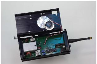
**3.** File a slot into the lower portion of the case as shown.
