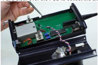
**4.** Carefully remove the IC U101 by gently prying it up on one end at a time.
