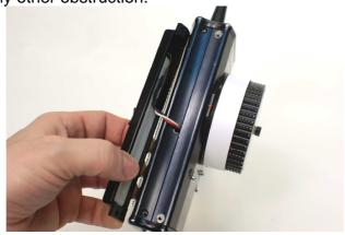
**8.** Place the Slider on the side of the **BarTech BFD Handset** with the slider stopper at the top as shown.
