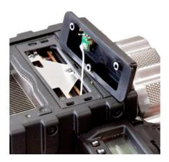
**Attach** the Range Extender for Red Epic<sup>™</sup> using the screws provided with the kit using a small (PH0) Phillips screwdriver.
