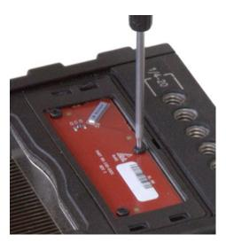
**Lift up** the Antenna board and carefully unplug the U.FL Antenna connector cable from the Antenna board.
