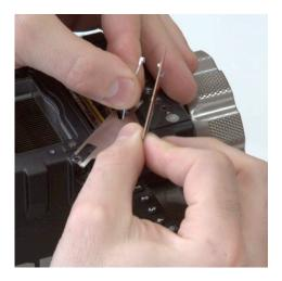
**Reposition** the U.FL Antenna cable to the right side of the metal plate.
