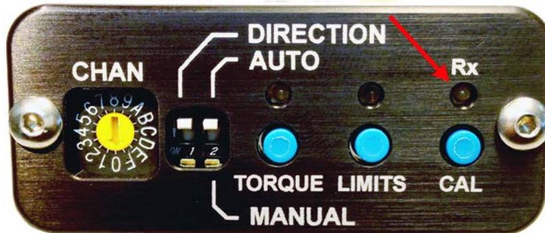
The **Rx** light is solid Red if the **fSTOP Wireless V2-1** is not communicating with the **BFD Handset**.
