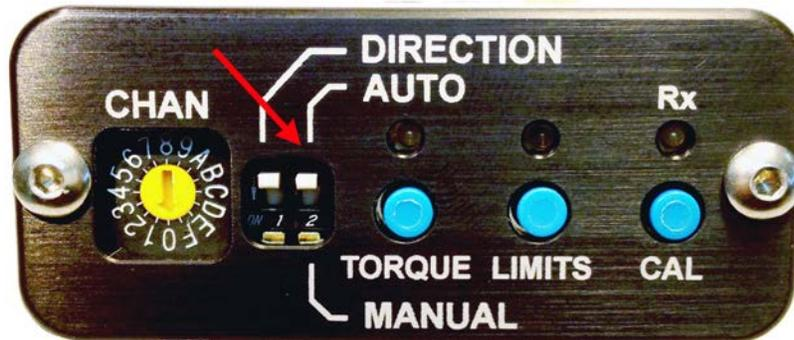
For lenses with no or soft end stops (most SLR lenses).
