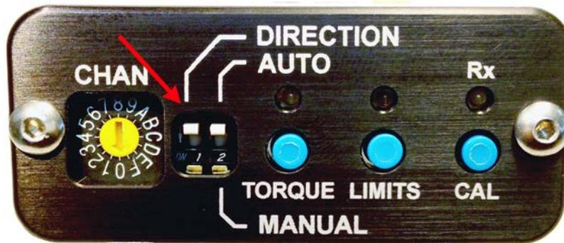
The **DIRECTION** Switch on the **fSTOP Wireless V2-1** sets the direction of travel of the motor. Toggling the direction switch will recalculate the position and slowly move the motor to the new position.
