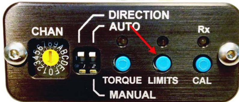
The **LIMITS** button is used to limit the travel of the motor between 2 user defined positions. When the limits are set the position of the focus knob on the **BFD Handset** is recalculated to the corresponding position between the 2 limits set by the user, i.e. fully clockwise will move the motor to one limit and fully counterclockwise will move to the other limit.
