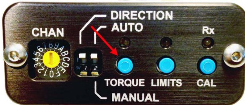
The **fSTOP Wireless V2-1** allows for the user to set the desired torque for the motor control. Generally the increased torque will allow for more accurate control on stiffer lenses, however there is a trade-off with increased noise generated by the motor.
