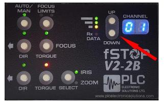
c. The focus wheel on the **BFD Handset** controls the focus motor on the **fSTOP V2-2B BarTech Receiver**. If you have the **BarTech Handset Iris Upgrade**, the additional slider will control the iris motor.
