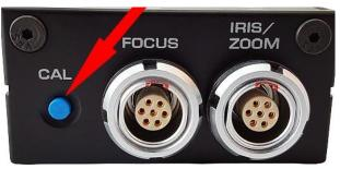
b. When the button is depressed and released it will reset the unit. The motors will then start their calibrate functions again immediately if in automatic calibration mode. If focus is in manual calibration the unit will be ready for settings in manual calibration mode. Limits will also be erased.
