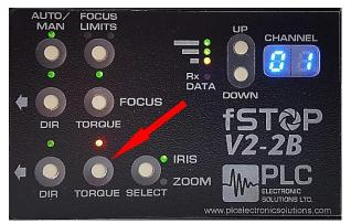
d. The torque is set and saved into memory. The torque light will change color to indicate the current torque setting:
