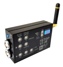
a. Attach the Antenna (PLC477-0012) to the **fSTOP V2-2B BarTech Receiver** (PLC955-0029).
