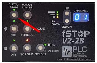
b. Ensure that the torque is set to the minimum usable setting before connecting the motor to a lens. See section **3.2.3.2. Setting Focus Torque**.
