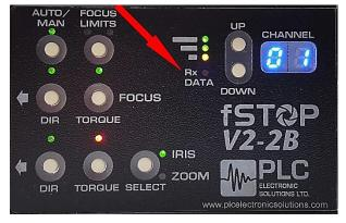
The signal lights indicate the strength of the signal being received, all lights 3 indicating a good signal and 1 yellow light indicating poor signal strength.
